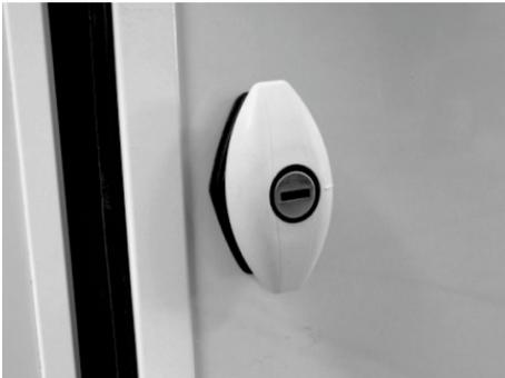
Fig. 19: Service compartment lock
