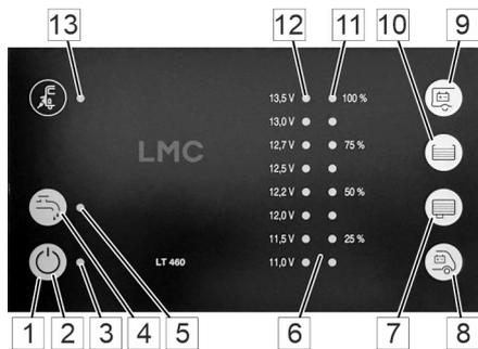
Fig. 55: Operating and control panel LT 460 A
