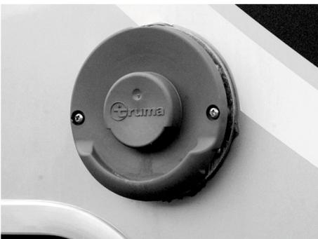
Fig. 74: Wall exhaust stack
