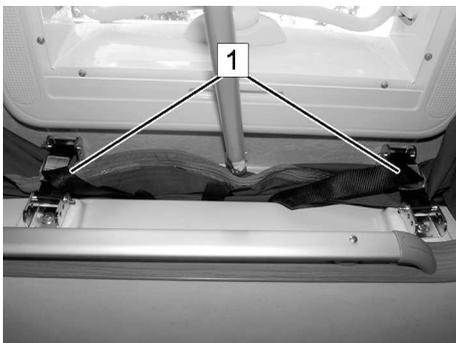
Fig. 133: Roof locking mechanisms
