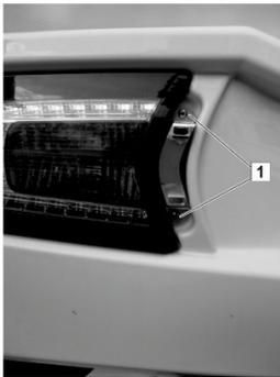
Fig. 160: Reattaching the rear lamp assembly
