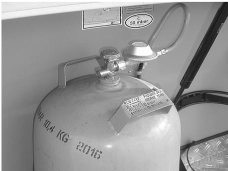
Fig. 86: Gas bottle with pressure reducing valve
