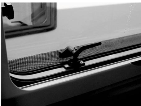
Fig. 88: Continuous ventilation
