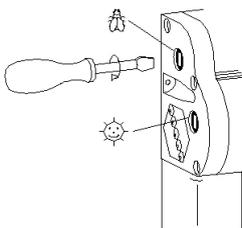
Use a screwdriver to re-tension the blind springs.
