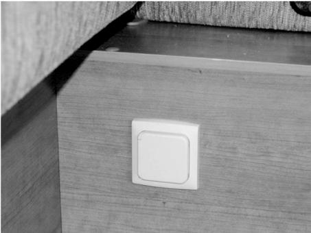
Outlets for the connection of small appliances when an external power supply is connected can be found at various locations in the vehicle interior, depending on the model and selected equipment (the picture shows an outlet in the support of the sitting area).
