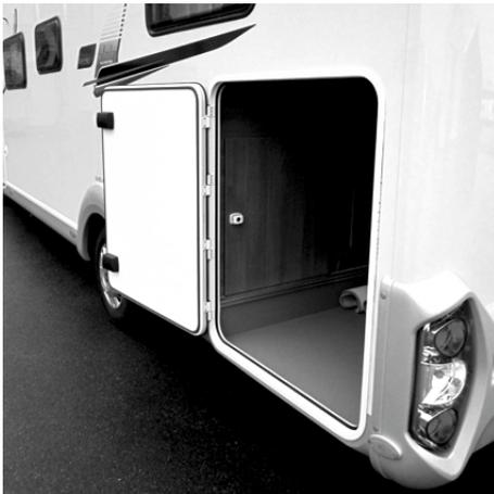
Depending on the model and selected equipment, hatches are located on the outside of the caravan. e.g.: accesses to rear external storage locker, hot water tank, to small storage compartments (for vehicle accessories, tools, car jack) and for the toilet waste holding tank.
