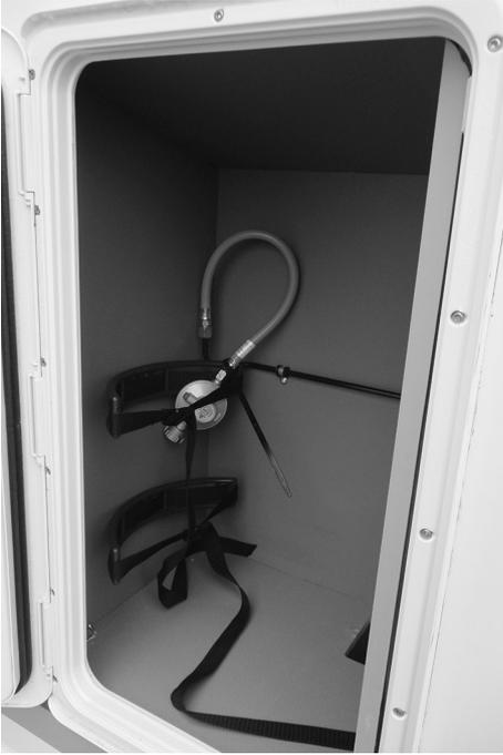
Fig. 65: Example of a gas bottle locker
