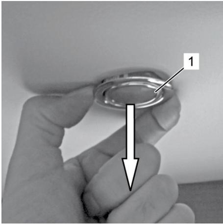
Fig. 155: Pull out the LED
