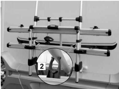
Fig. 25: Folding up the bicycle carrier
