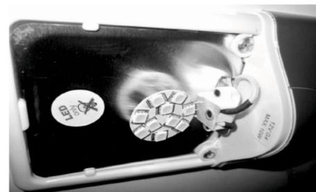
Fig. 153: Inserting the LED light
