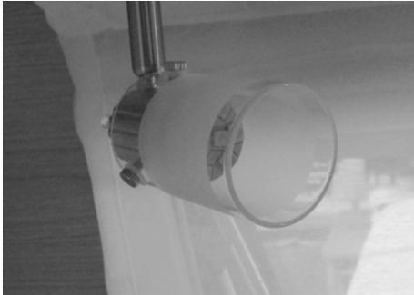
In the interior, above the bench and in the sleeping area, there is a track light system with 12 V LED spotlights. Those can be rotated, pivoted and adjusted, allowing all areas to be well illuminated (for use see → "Arranging the lights" section).
