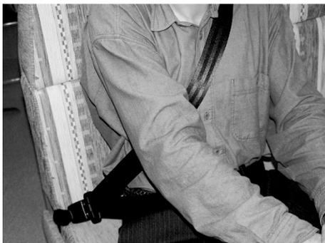
Fig. 11: Three-point safety belt
