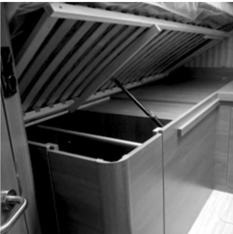
Fig. 42: Gas pressure spring
