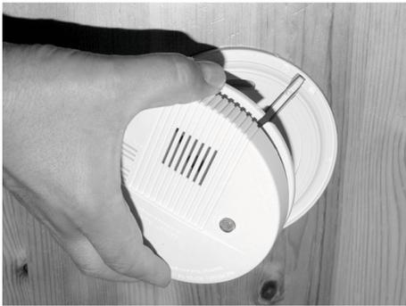
Fig. 161: Removing the housing
