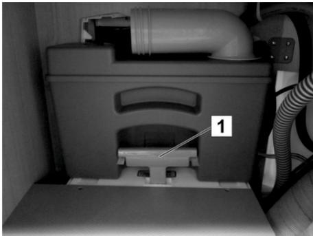
Fig. 140: Waste holding tank in the disposal shaft
