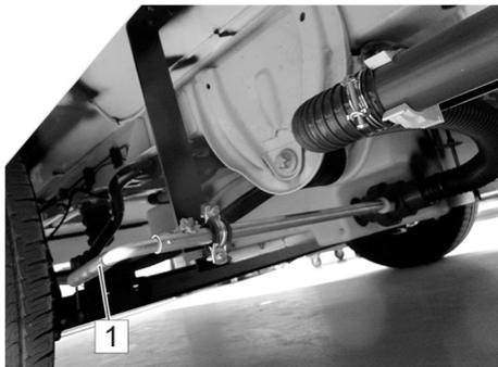
Fig. 83: Linkage assembly for drain valve, example
