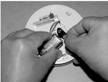
Fig. 162: Replacing the block battery
