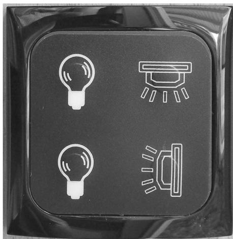
One or two switches are installed at convenient height in the entrance area. They control the various sources of light from inside and outside of the vehicle, permitting lighting the interior before entering the vehicle body.
